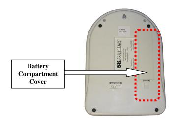
Figure 1: Battery Compartment Cover
