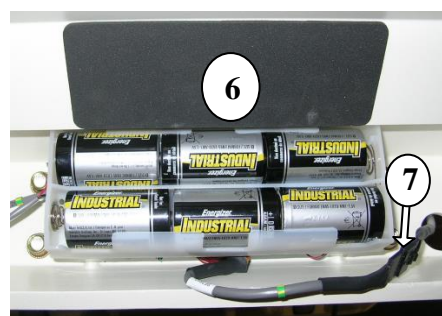
Figure 2: Display Cable Connector and Battery Compartment Cover
